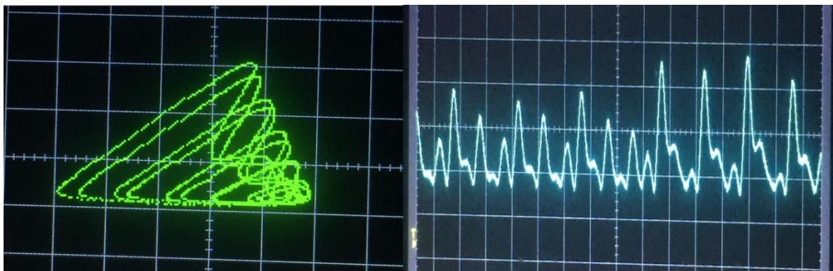
Figure 17: Experimental oscilloscope pictures of Colpitts oscillator: 2D projection of the chaotic attractors for (x vs z) on the LHS and time series (RHS) for  $R_1 = 36\Omega$ .
