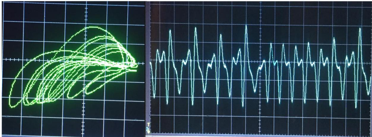
Figure 13: Experimental oscilloscope pictures of Sprott I oscillator: 2D projection of the chaotic attractors for (x vs z) on the LHS and time series (RHS) for  $R_2 = 61.9k\Omega$ .
