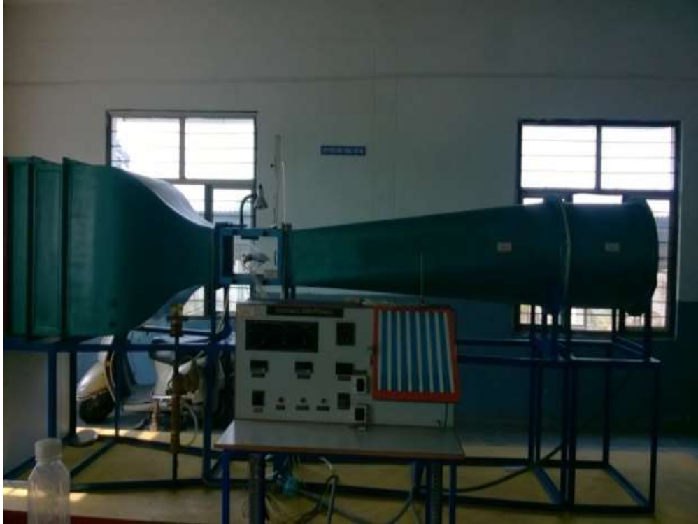
Fig. 4 low speed wind tunnel used for testing
