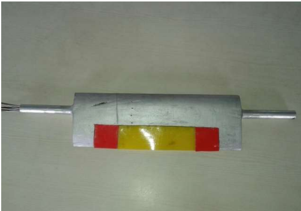
Fig. 5 Flex foil prototype used in wind tunnel testing.
