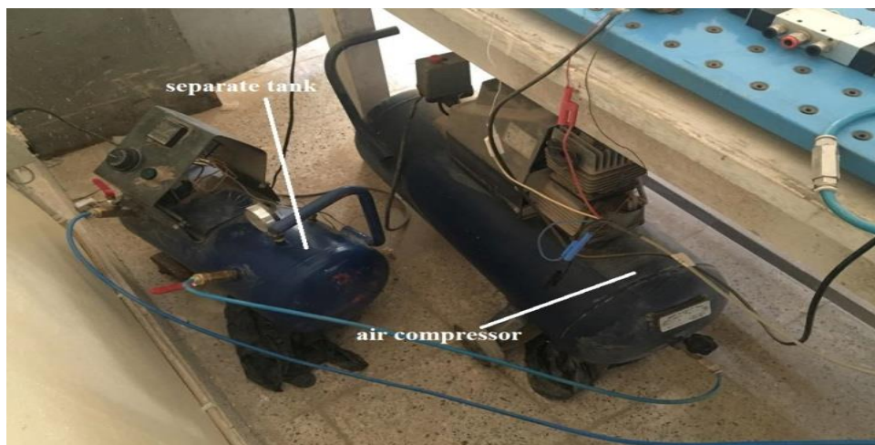
Fig. 3. Air compressor and the separate tank
