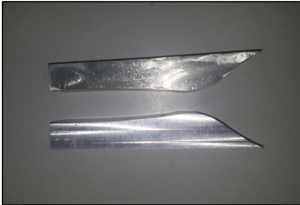
Fig 3: Convergent-Divergent Nozzle Profile
