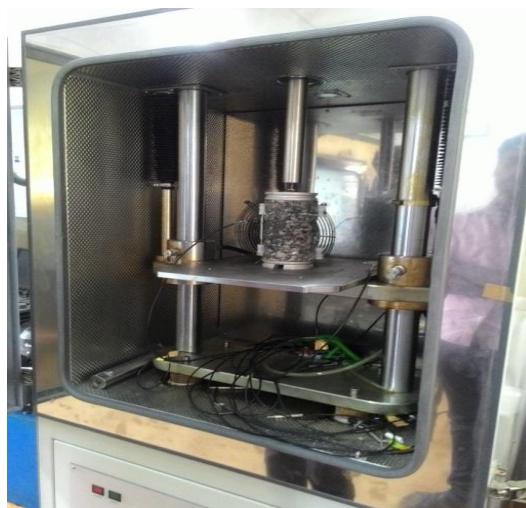
Fig.8.1: Dynamic Modulus Test Setup
