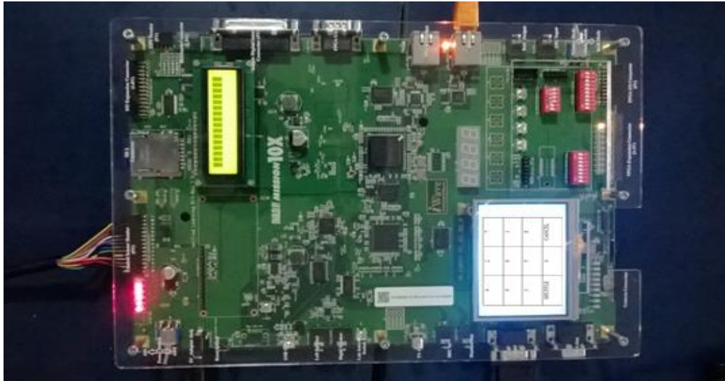
Fig.4. SHUFFLED KEYPAD USING ARM PROCESSOR
