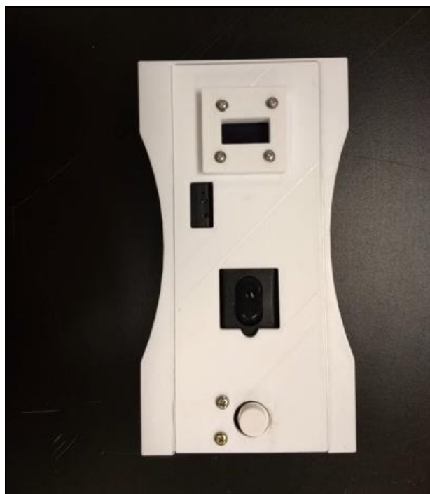
Fig. 3: Top view of the sensor system in 3-D printed housing
