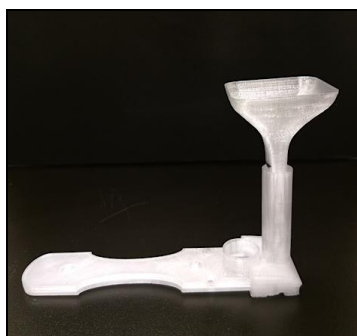
Fig. 2: Side view of the 3-D printed saliva funnel, collection device, and test strip components
