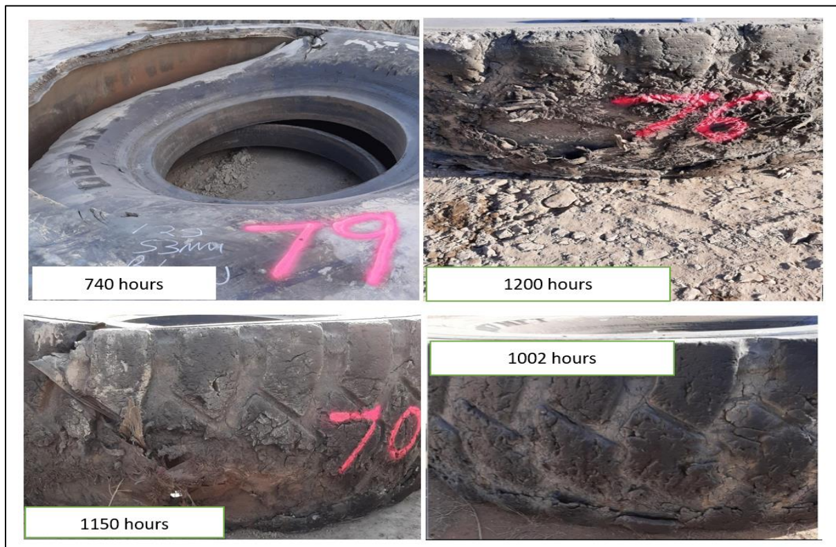
Figure 19: Tyres Failure Modes
